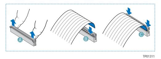
Figure 28. Installing the Flat Flex Cable to the Floppy Drive
